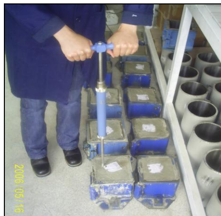
Figure 1. Penetration application to fresh concrete mortar
