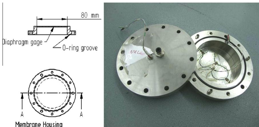
Fig. 4. Design of the null pressure sensor.
