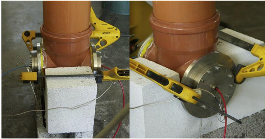
Fig. 7. Arrangements for the measurement of lateral concrete pressure.
