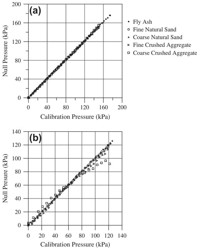
Fig. 6. Null pressure as a function of applied pressure, response to aggregate pressure. (a) Large null sensor. (b) Small null sensor.
