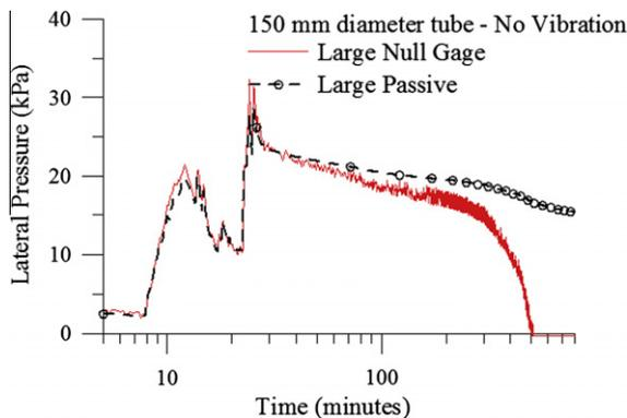
Fig. 9. Lateral concrete pressure as a function of time, Test 2.
