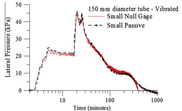
Fig. 10. Lateral concrete pressure as a function of time, Test 3.
