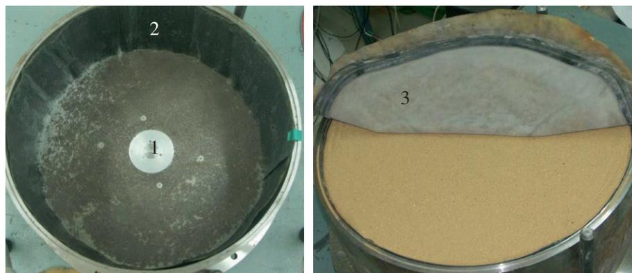
**Fig. 2.** Pressure vat. 1 – Flush pressure transducer. 2 – Friction reduction tarp. 3 – Vat seal.
