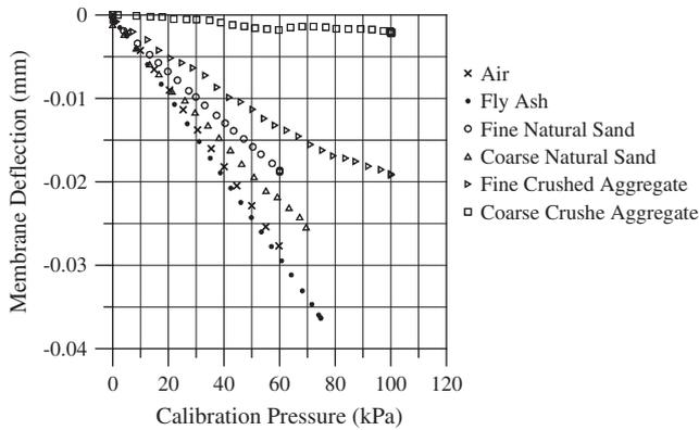
Fig. 3. Membrane deflection as a function of applied aggregate pressure.
