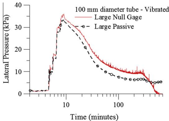
Fig. 8. Lateral concrete pressure as a function of time, Test 1.
