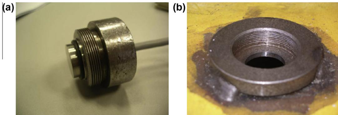
Fig. 4. Pressure cell with the washer and the socket welded to the formwork.
