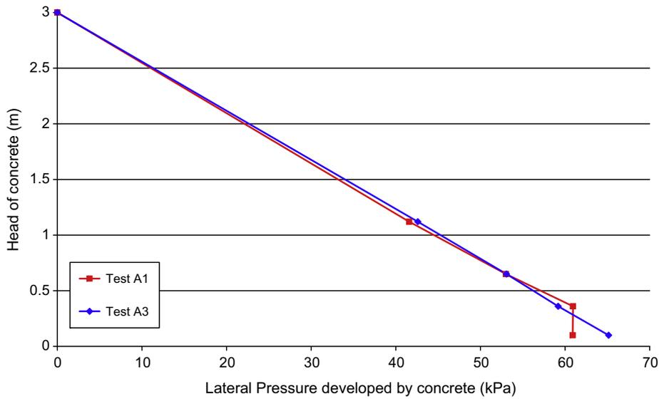
Fig. 5. Envelope of concrete lateral pressure.
