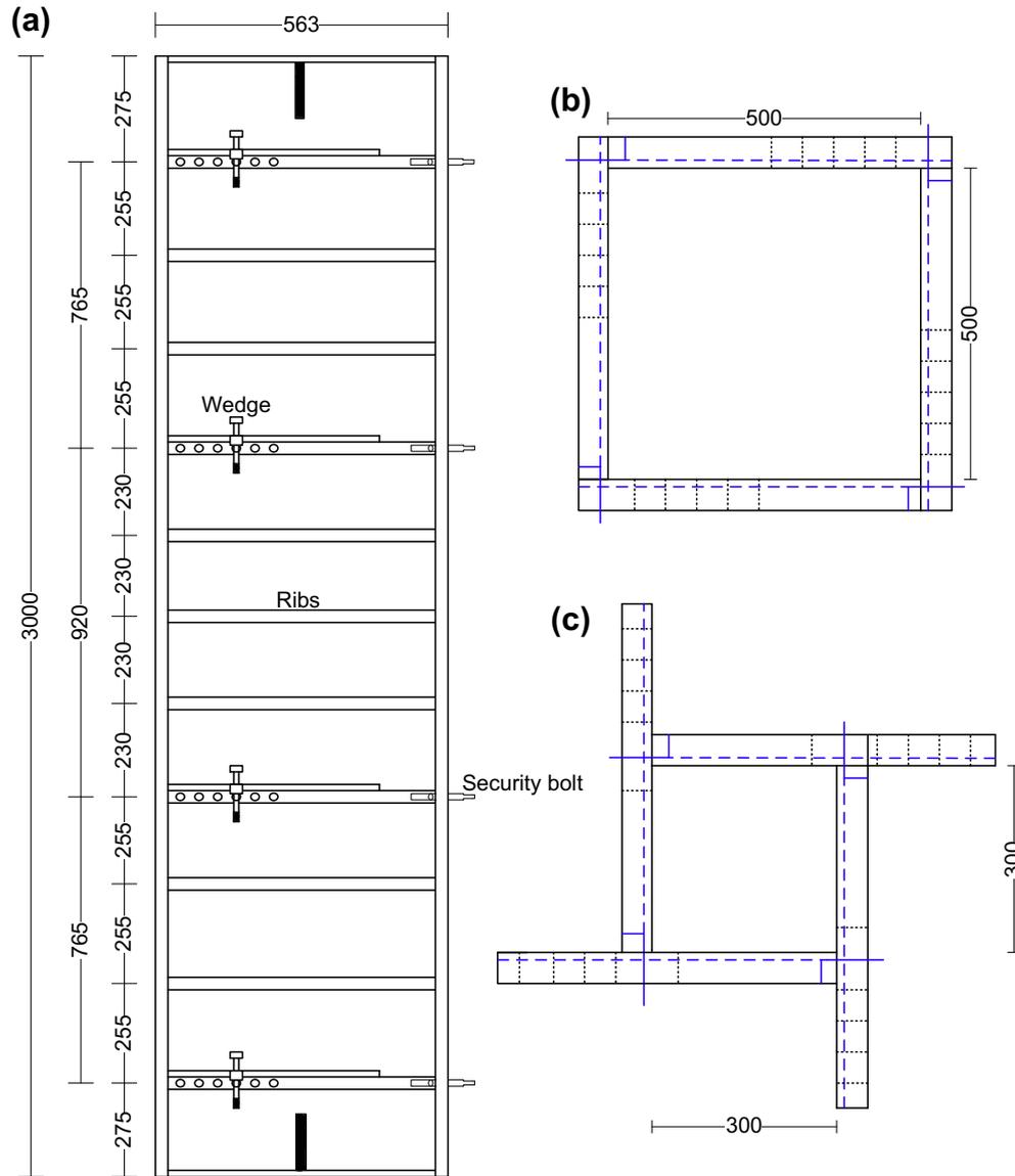
Fig. 1. Square formwork plot (mm).
