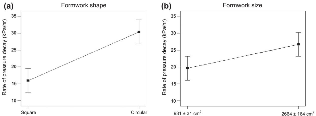
Fig. 8. Main effect plot for initial rate of pressure decay significant parameters.
