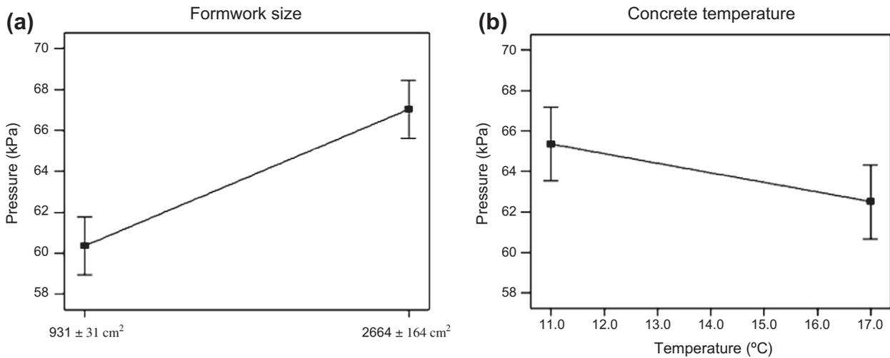
Fig. 7. Main effect plot for lateral pressure significant parameters.
