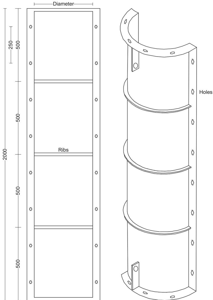
Fig. 2. Circular formwork plot (mm).
